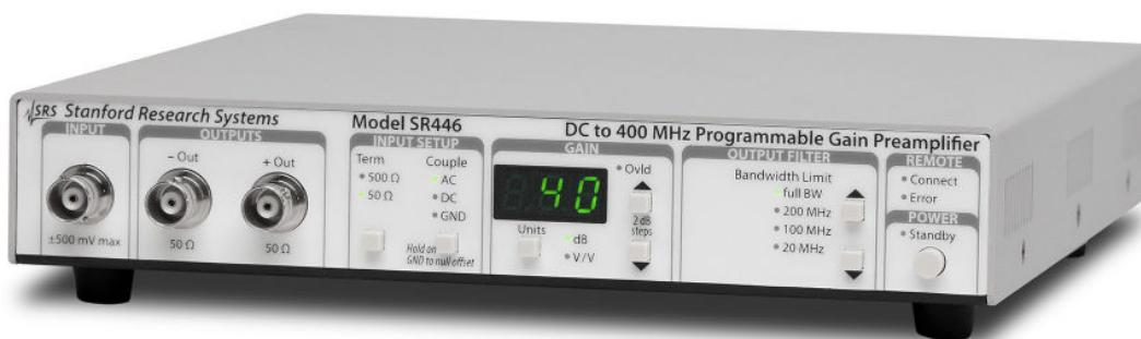
The SR446 is a single-channel, 400MHz bandwidth voltage preamplifier with 21 programmable gains from 1 to 100 (+0 dB to +40 dB with 2 dB steps). It also includes four programmable low-pass filters, with settings of full bandwidth, 200 MHz, 100 MHz and 20 MHz. There are two output channels which offer complimentary outputs (inverting and non-inverting) that can be used separately, or together as a differential output.
